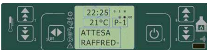
fig. 34 control panel - cooling wait before restart
