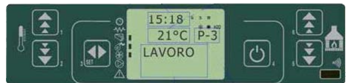
fig. 28 control panel - operating condition
