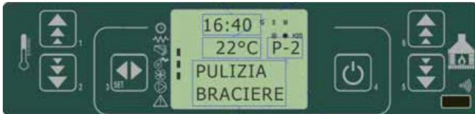
fig. 31 control panel - brazier cleaning mode
