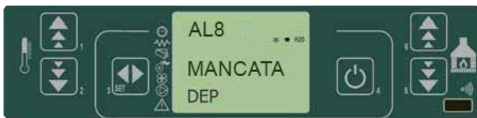
fig. 41 control panel - auger safety pressure switch alarm
