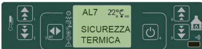
fig. 42 control panel - general thermostat alarm
