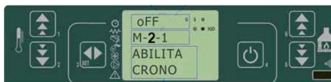
fig. 20 control panel - enabling chronothermostat functions
