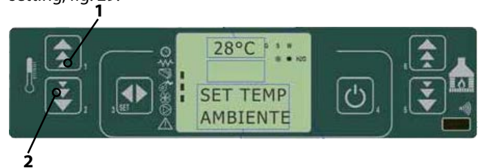
fig. 29 control panel - room temperature change
