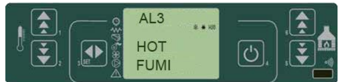
fig. 38 control panel - flue gas overtemperature alarm
