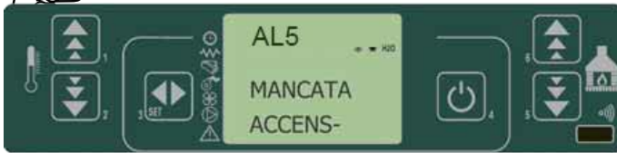
fig. 47 control panel - failed pellet ignition
