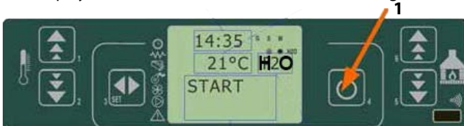
fig. 27 control panel - ignition
