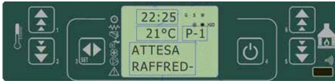
fig. 31 control panel - cooling wait before restart
