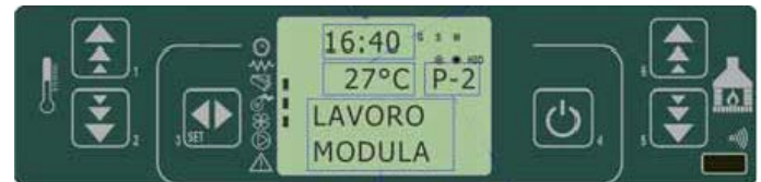
fig. 27 control panel - set temperature modulation
