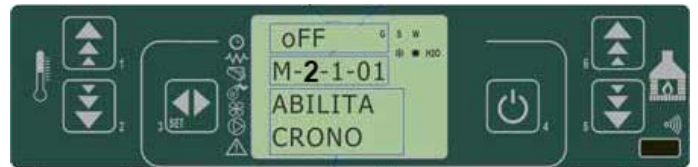
fig. 17 control panel - enabling chronothermostat functions
