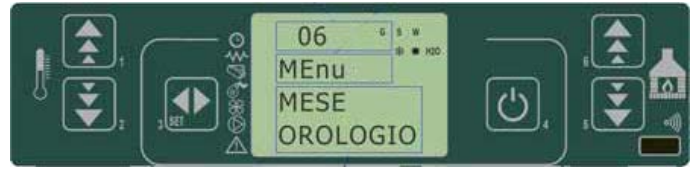
fig. 16 control panel - time and date setting
