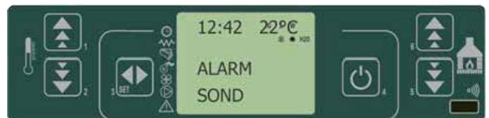
fig. 33 control panel - flue gas temperature sensor alarm
