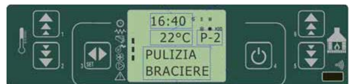
fig. 28 control panel - brazier cleaning mode
