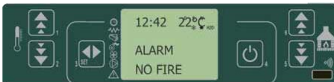
fig. 36 control panel - extinction during operation alarm
