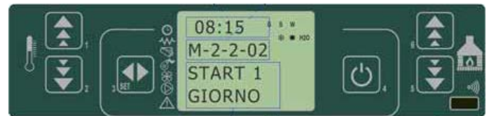
fig. 18 control panel - daily programming
