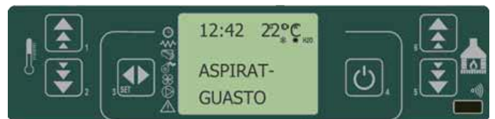
fig. 39 control panel - flue gas extraction fan alarm
