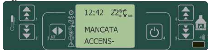
fig. 40 control panel - failed pellet ignition
