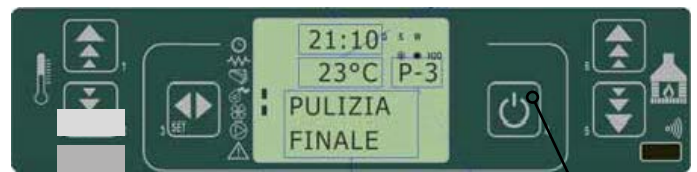
fig. 29 control panel - final cleaning
