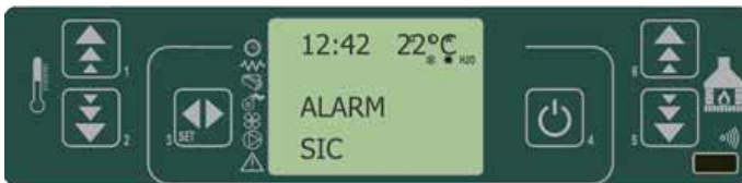
fig. 38 control panel - general thermostat alarm
