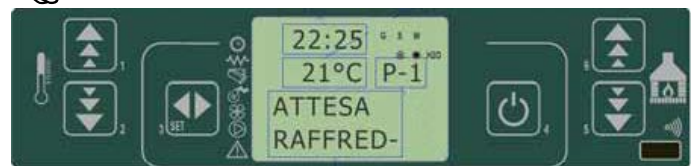
fig. 31 control panel - cooling wait before restart
