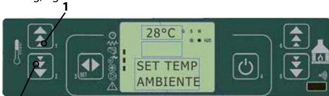
fig. 26 control panel - room temperature modification
