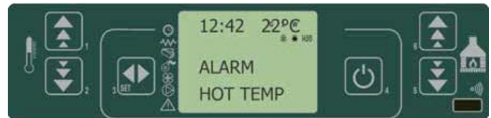
fig. 34 control panel - flue gas overtemperature alarm
