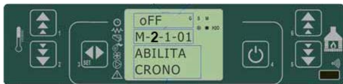
fig. 17 control panel - enabling chronothermostat functions
