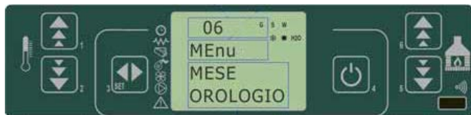
fig. 16 control panel - time and date setting
