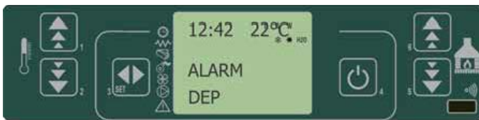
fig. 37 control panel - auger safety pressure switch alarm
