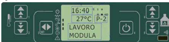
fig. 27 control panel - set temperature modulation
