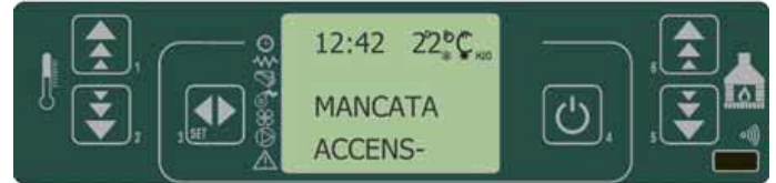
fig. 40 control panel - failed pellet ignition
