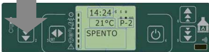
fig. 33 control panel - switch-off
