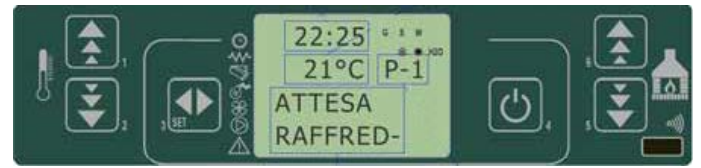
fig. 34 control panel - cooling wait before restart
