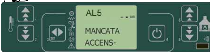
fig. 47 control panel - failed pellet ignition
