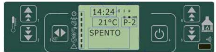
fig. 17 control panel off
