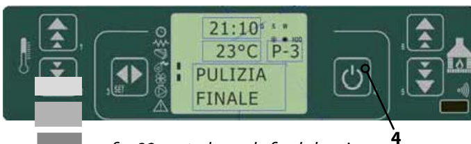
fig. 32 control panel - final cleaning
