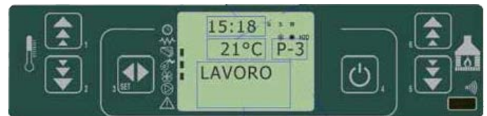
fig. 28 control panel - operating condition
