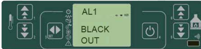
fig. 48 control panel -power failure
