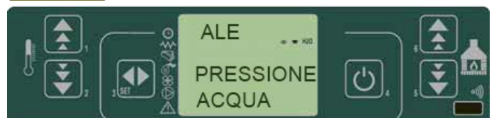
fig. 46 control panel - water pressure
