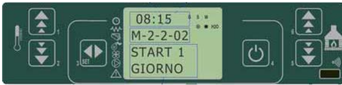
fig. 21 control panel - daily programming
