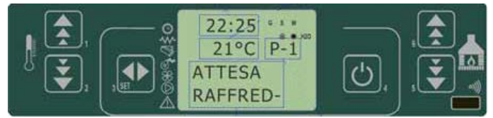
fig. 34 control panel - cooling wait before restart
