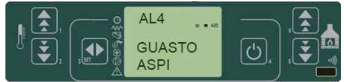
fig. 43 control panel - flue gas extraction fan alarm
