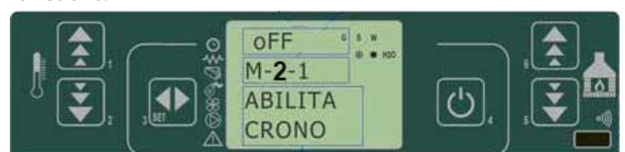
fig. 20 control panel - enabling chronothermostat functions
