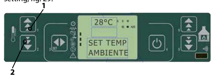
fig. 29 control panel - room temperature change
