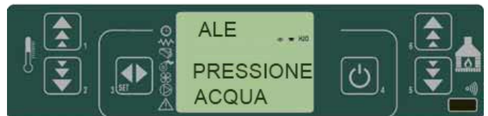
fig. 46 control panel - water pressure
