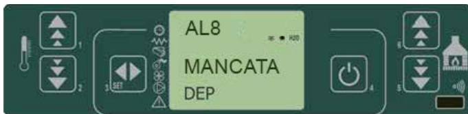
fig. 41 control panel - auger safety pressure switch alarm
