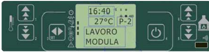
fig. 30 control panel - set temperature modulation
