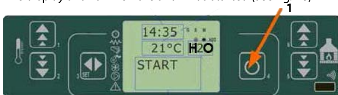
fig. 27 control panel - ignition
