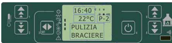
fig. 31 control panel - brazier cleaning mode
